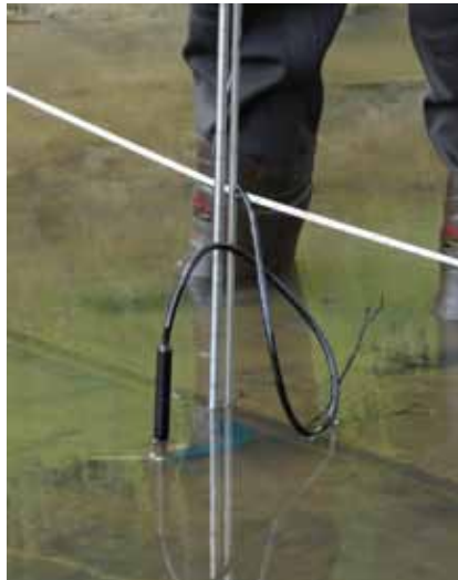
Figure 5. LGS staff conducting a Flow Tracker® survey of Beaver Bayou near Wax Road in Baton Rouge, Louisiana on June 20, 2013.
