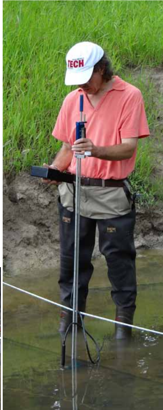
Figure 5. LGS staff conducting a Flow Tracker® survey of Beaver Bayou near Wax Road in Baton Rouge, Louisiana on June 20, 2013.
