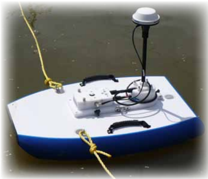
Figure 3. Above is a close up view of the River Surveyor. Box towards bow end (left) is power source, the tower near stern (right) is global positioning system (GPS) unit used for locating boat on universal grids (latitude-longitude or State Plan Coordinates (UTM)).
