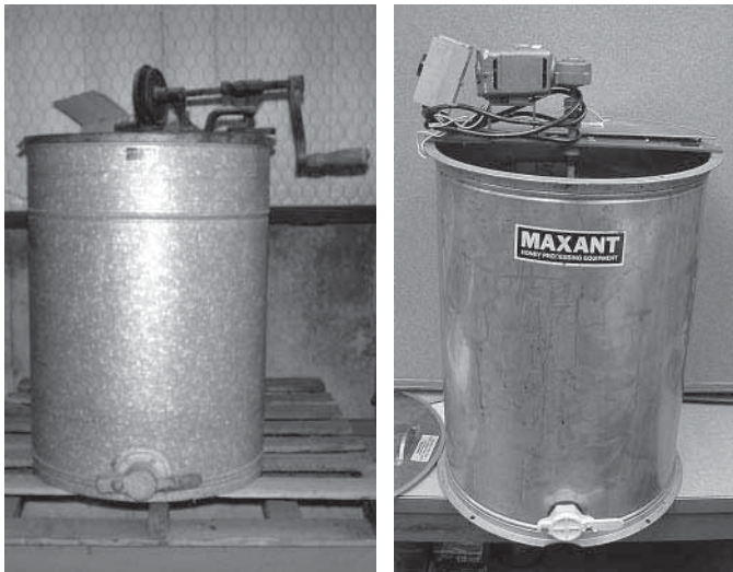
Figure 31. Old two-frame hand cranked honey extractor (left) and new three-frame electric honey extractor (right).
