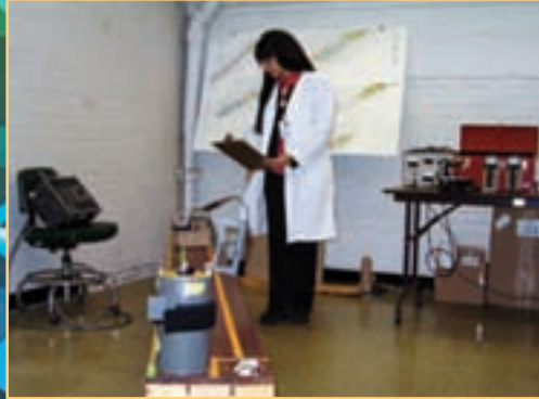
RSO manager Mary Haik carries out a regular calibration on a radiation survey meter using a cesium-137 calibrator.
