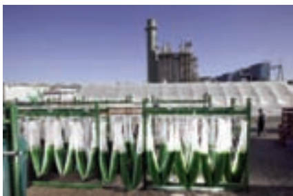
Algae, shown here growing at the Redhawk power plant near Phoenix, have been reported to absorb carbon dioxide and produce 5,000 gallons of biodiesel an acre each year (Sengupta and Pike, 2009).
