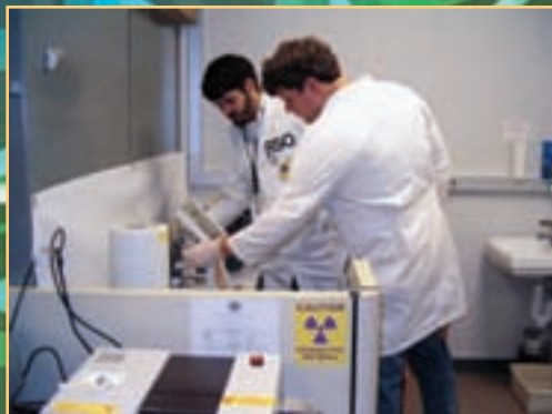
Radiation specialist Cade Register and technical assistant Charlie Wilson perform a leak test on a sealed radioactive source.
