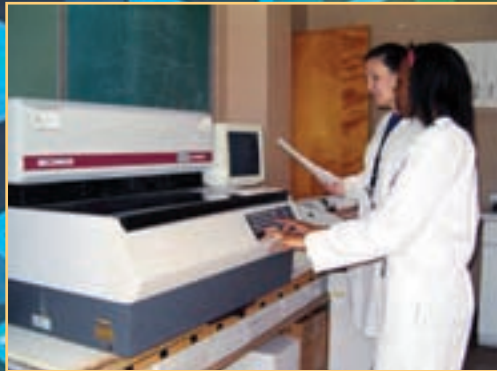
Assistants Rebecca Hill and Dana Lewis count the swipes from routine radiation laboratory surveys using a liquid scintillation counter.
